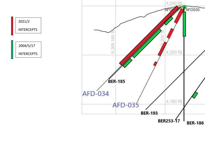
AFD holes are 2021/2 diamond drilling – voids not shown. BER holes are 2004/5/17 RC drilling.
