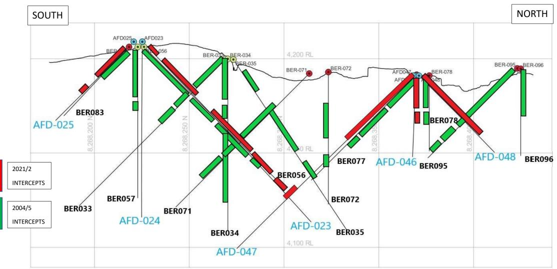
AFD holes are 2021/2 diamond drilling – voids not shown. Results awaited AFD-024 BER holes are 2004/5 RC drilling.
