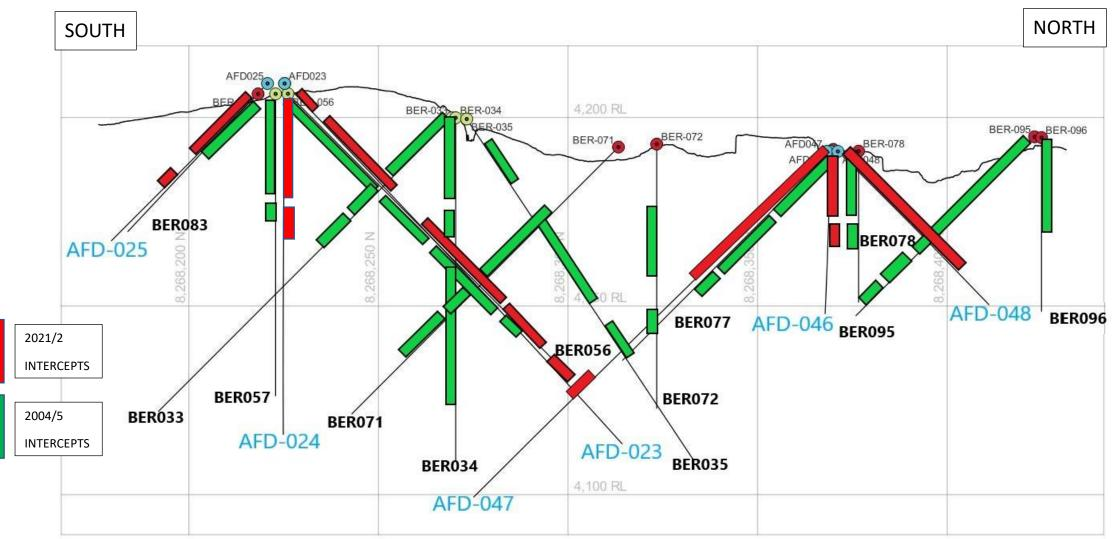
AFD holes are 2021/2 diamond drilling – voids not shown. BER holes are 2004/5 RC drilling.
