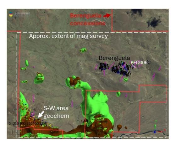
GREEN isosurfaces are areas with high magnetic susceptibility usually indicating the presence of magnetite as an alteration mineral in intrusives.
