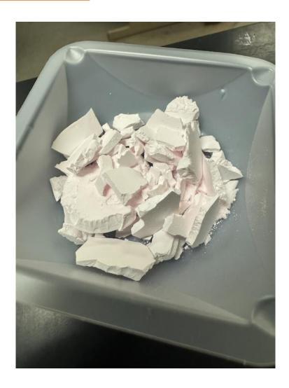
Figure 1. Battery grade crystallized MnSO<sub>4</sub> prepared by KCA from Berenguela composite sample RD4LOWA.
